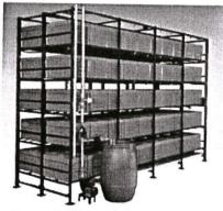
Curing process starts when the water is pumped up through the piping system and dispersed mist via sprinklers on top of each HDPE crates, where the treated and shredded vegetable/agricultural wastes are placed. It allows beneficial microbes to multiply which will convert it to matured compost. The equipment can produce 200 kg of compost per day.
