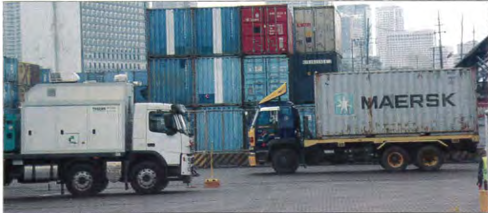
A container van undergoing X-ray scanning.
